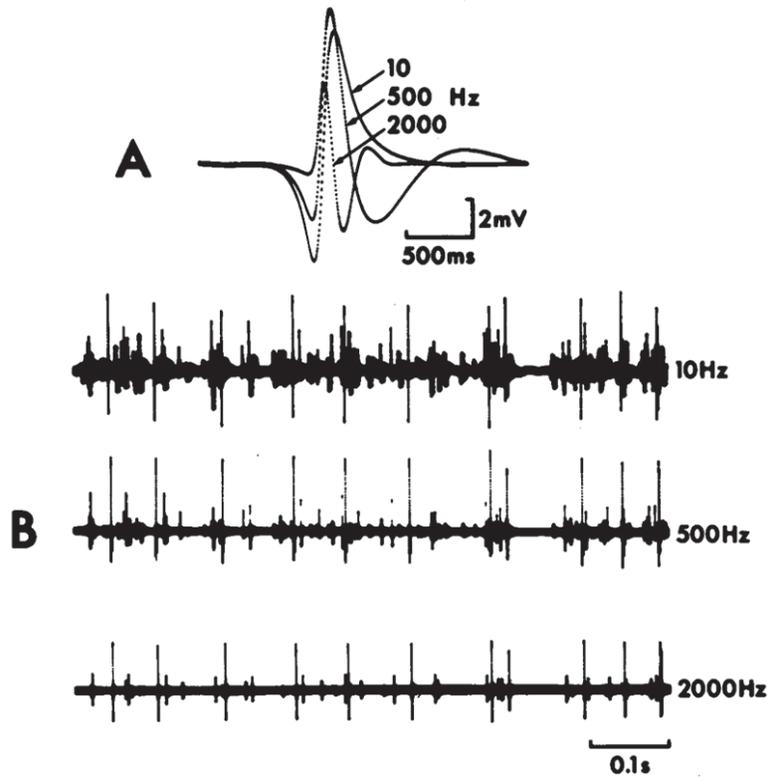
**Fig. 2.6.** Effect of filtering. A - on the shape and amplitude of the single fiber action potential. B - on the background activity.
