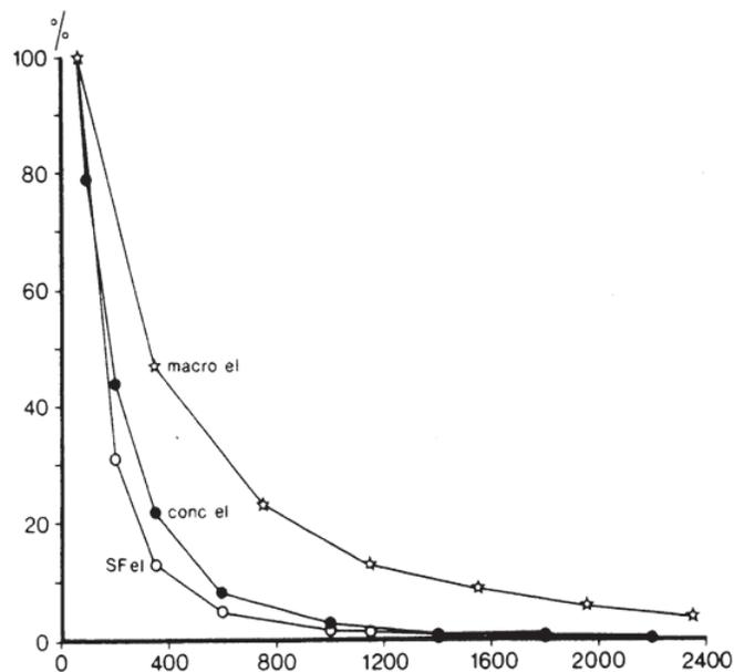
**Fig. 2.2.** Relative peak-to-peak amplitude of a simulated SFAP at different distances from the fiber surface as measured by a SFEMG (square), concentric needle (round) and Macro (star) EMG electrode. The SFEMG AP was filtered with a 500 Hz high-pass filter. The APs in CNEMG and Macro EMG were not filtered. (Modified from [Stålberg, 1983] with permission.)
