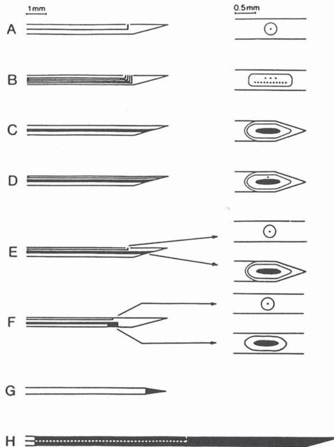
**Fig. 2.3.** EMG electrodes. A - single fiber EMG electrode with one recording surface. B - single fiber multielectrode. C - concentric needle electrode. D-F - different types of dual electrodes. G - monopolar electrode. H - Macro EMG electrode (From [Stålberg, 1986] with permission.)
