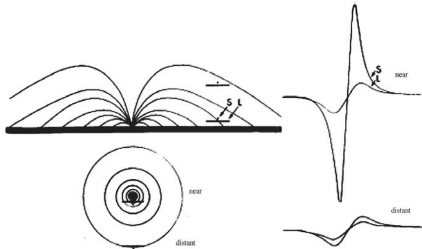
**Fig. 2.1.** The electrical field around a muscle fiber recorded with a small (S) and a large (L) electrode surface. The large electrode shunts the isopotential lines at short fiber - electrode distances, but less so at longer distances. Thus at a short distance the large electrode records a lower amplitude of the AP than the small electrode.
