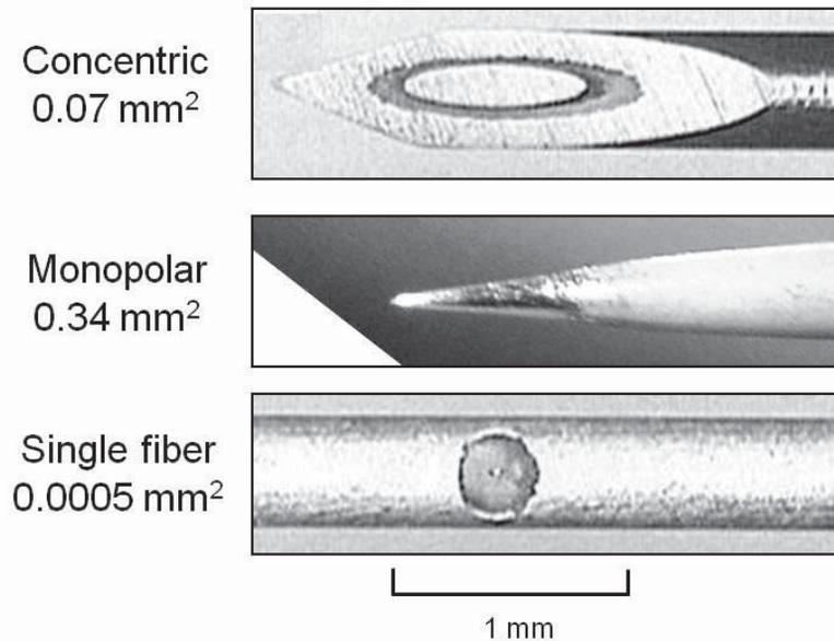
**Fig. 2.4.** Microphotographs of three types of EMG electrodes. (Figure courtesy S. Nandedkar)
